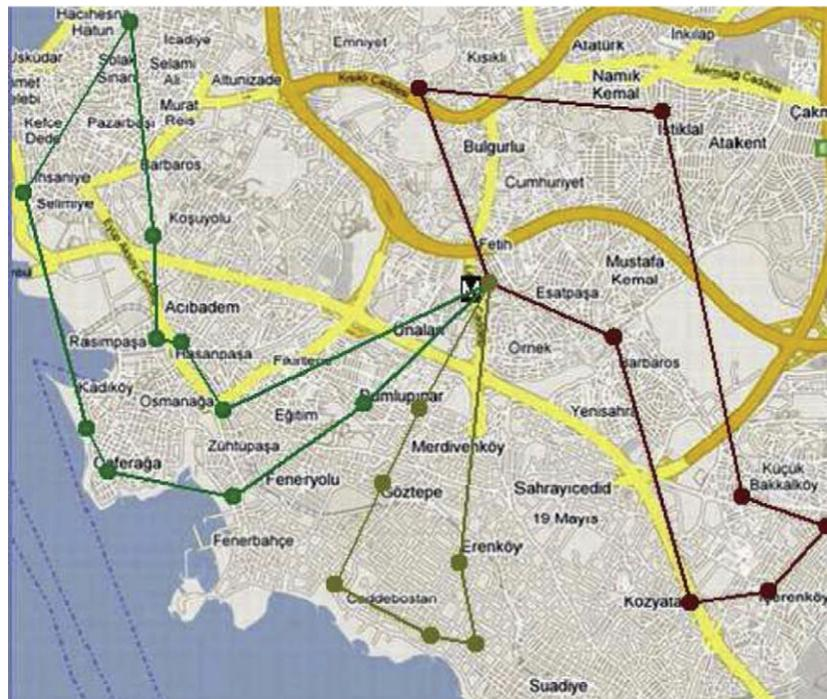
**Fig. 3.** Supermarket food distribution optimization of repartition and routing for 3 vehicles, for a particular store, using an imbedded double simulated annealing. From A. Erbaş, M.S. Thesis (Koç University, Istanbul, 2007).
